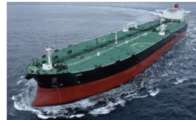
Sifa VLCC In January 2011, we delivered this 317,000 dwt very-large crude oil carrier to Oman Shipping Company. Sifa is the industry's first VLCC equipped with a ballast water treatment system. The system is capable of handling approximately 100,000 metric tons of ballast water in 20 hours, the equivalent of 50 Olympic-sized swimming pools.
