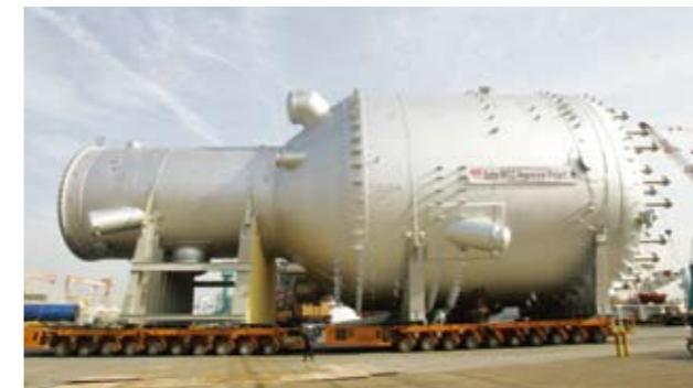
RFCC reactor shipment
