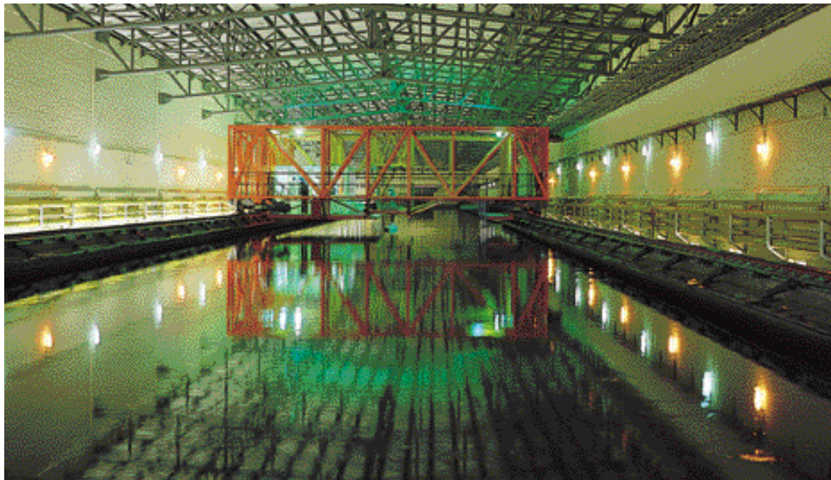
Towing Tank for Modelship Test
