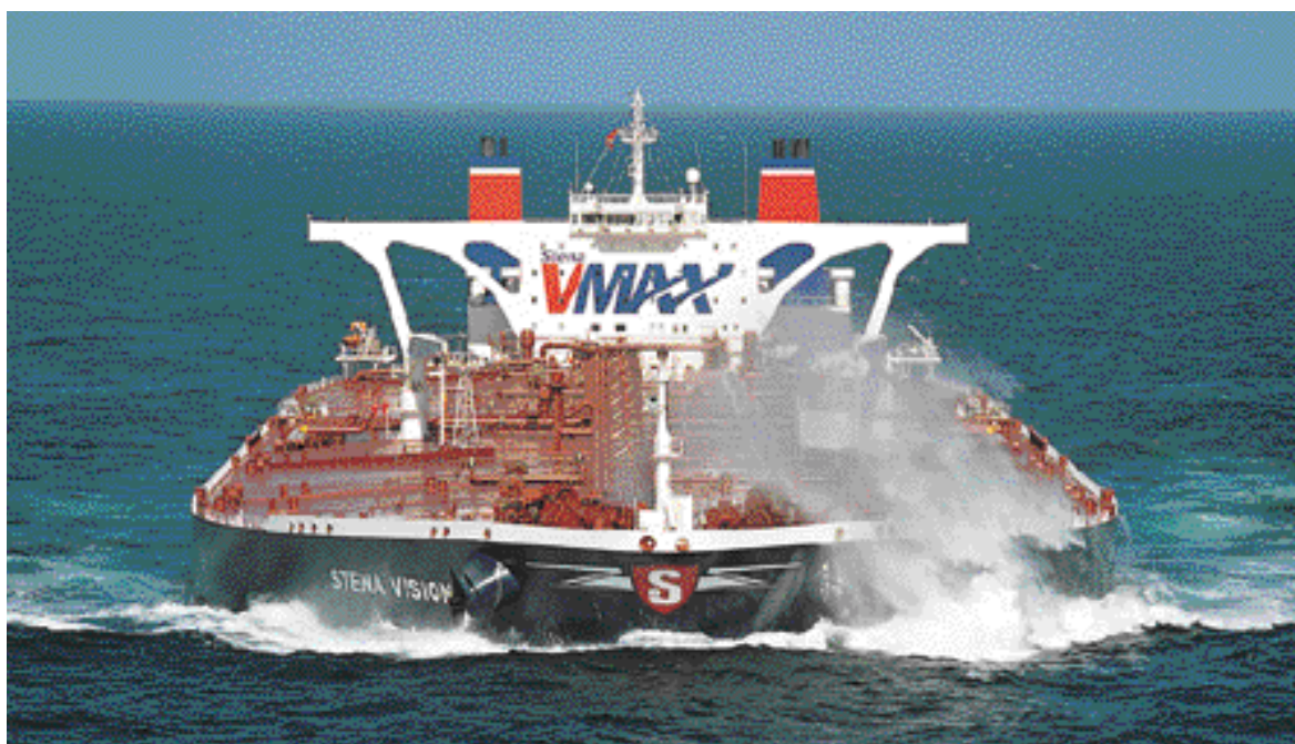
The Stena Vision, a 315,000 DWT twin-skeg VLCC
