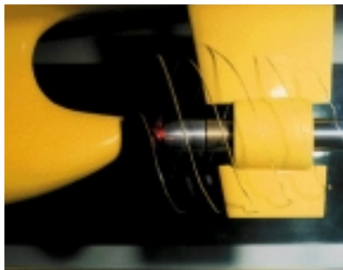
Propeller Cavation Test
